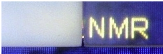
Fig. 3. Transparent property of the 60/40 (w/w) UPR/PEO–PPO–PEO blends: (left) UPR/EO30 and (right) UPR/EO80. The sample thickness is 2 mm and the two lightening words “NMR” are on the back of the two samples.
